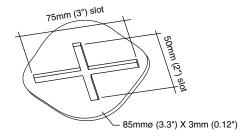
Figure 3 Insulation Support/Retainer
