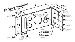
Figure 1 Slotted L-Plate
